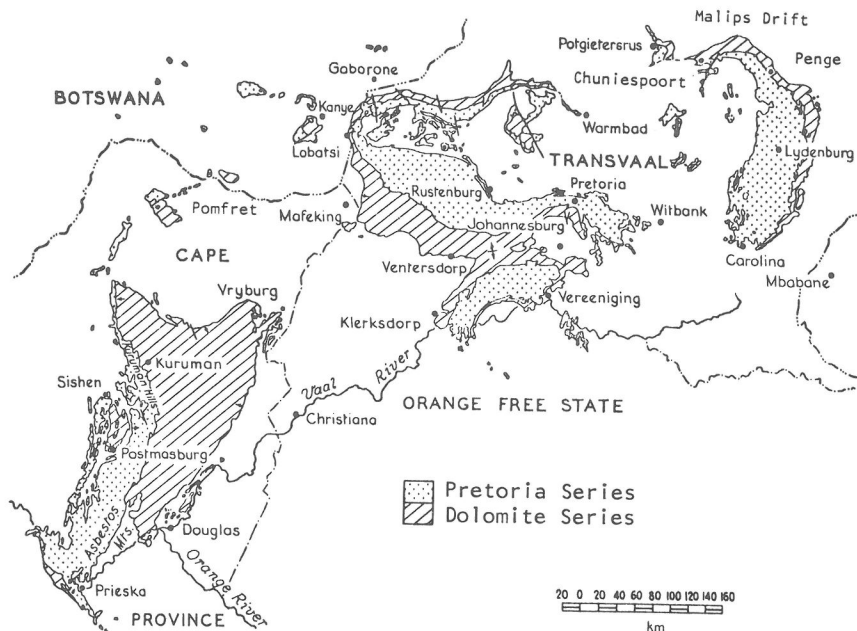
Figure 3. Index map of the crocidolite and amosite asbestos-bearing iron formations of the Transvaal and Cape Provinces of South Africa. After Truswell (1977).
